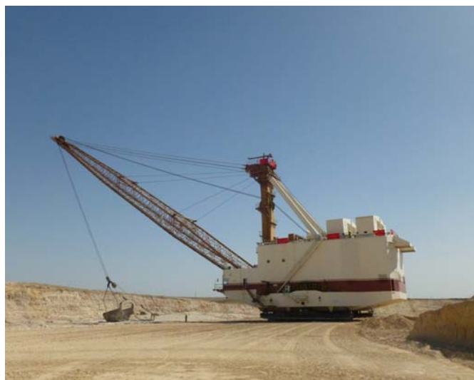
A dragline excavator at Khourigaba.
